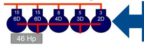
Increased Steps of Unloading Better Load Matching More Compressors Needed Increased Equipment Costs
