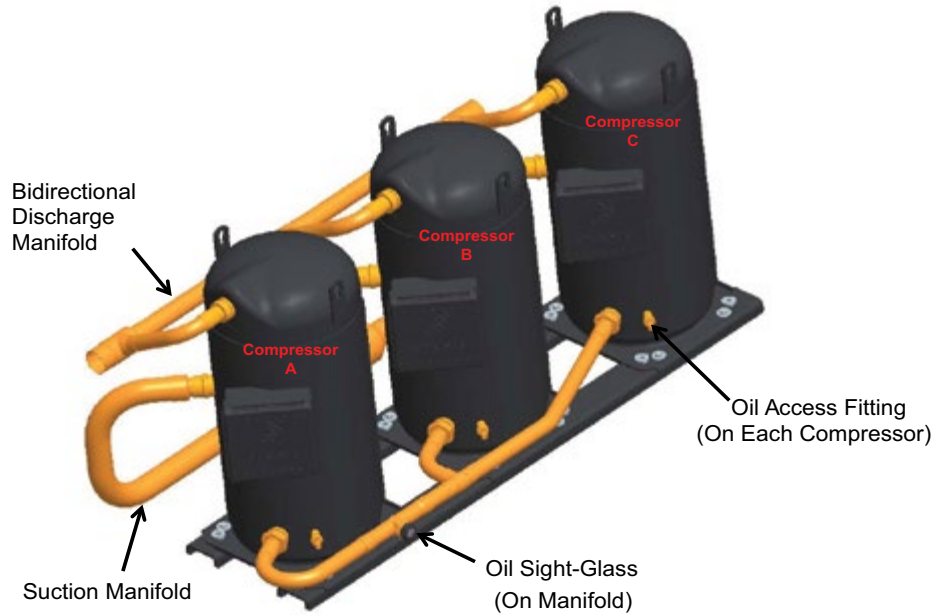
Figure 8 – Typical Braze Connected Trio with TPTL Oil Manifold
