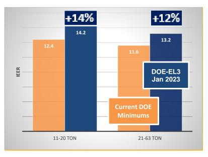
Figure 1: Department Of Energy Efficiency Levels Effective January 1, 2023 For Commercial Rooftops And Split Systems
