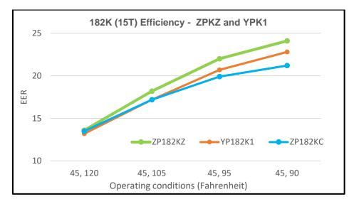
Figure 7: 12-15T Efficiency Comparisons – ZPKZ (improved R410A) and YPK1 (R32) versus ZPKC (legacy R410A)
