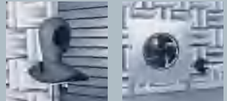
Room for precision noise measuring
